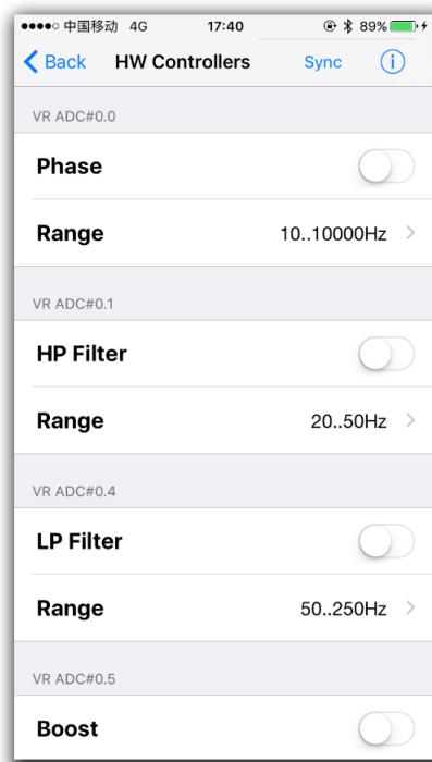
Fig 22. HW controllers window.
